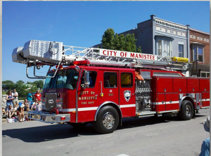
Ladder 651 – 1997 E-One Aerial Quint 70 foot ladder, 2000 GPM pump
