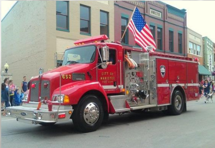
Engine 652 – 2004 Pierce Pumper 1250 GPM pump
